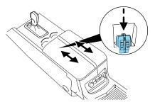
the backup slot, located in the rear of the center console utility compartment. Insert the IA key into the slot with buttons facing out and with key ring up. After inserting the IA key into the backup slot, use the START/STOP button and brake pedal to start your vehicle as usual. The vehicle should respond normally as long as the IA key is in the backup slot in the center console utility compartment. Once the vehicle is started, the IA key can be removed from the backup slot, if desired.
